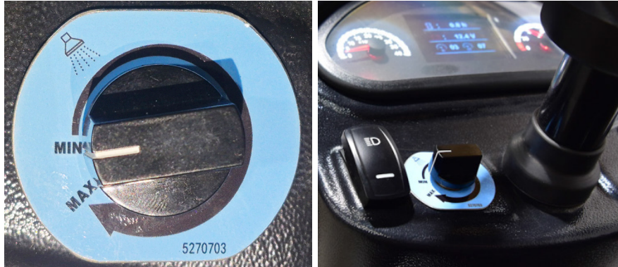
WATER PUMP CONTROL PANEL CLOSE-UP LEFT) AND LOCATION (RIGHT)
